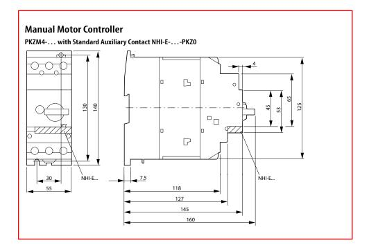
Dimensions are in millimeters.
