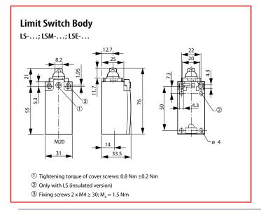
Dimensions are in millimeters.
